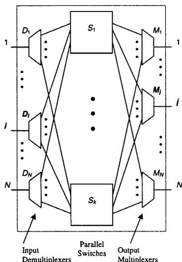
Fig. 2. Parallel switches.
