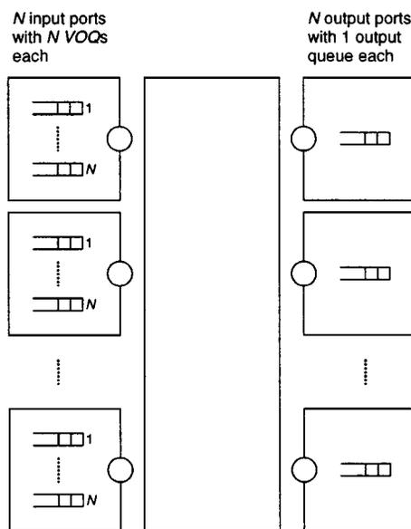
Fig. 1. Input–output-queued switch.
